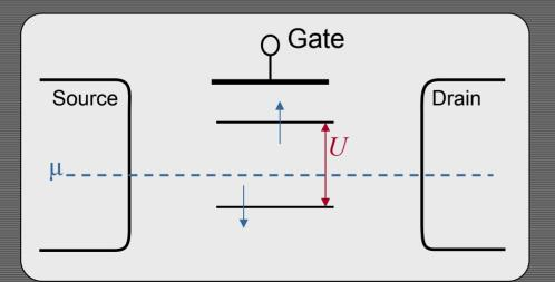
• For the diagram on the left, effectively the down spin level is filled first and the second electron, which will enter the up spin level, feels a charging energy of U = q/c. This charging energy, when large, creates an observable split in the spin levels and hence the observed coulomb blockade.
