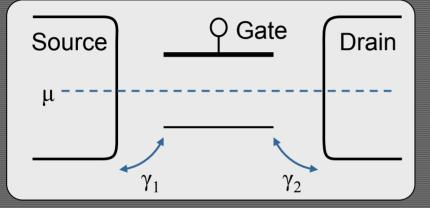
• For small U the single level device gives a conduction distribution and electron count as shown on the right. *Note*: The conductance peak has a width of  $\gamma_1 + \gamma_2 + 2U$ , where the electron charging energy is included twice
