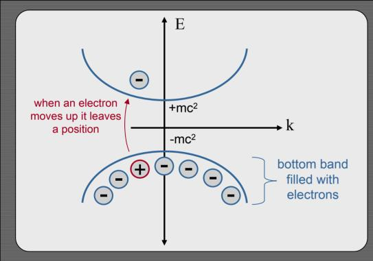
• Note however, that moving to the top band requires an energy equal to 2mc<sup>2</sup> (on the order of 1MeV)
