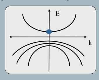
• ... If we were to examine the area right around the "dot" we would find that conduction band was formed of |s> orbitals and the valence band of |p> orbitals ( $|p_x>,|p_y>,|p_z>$  or in another notation |x>,|y>,|z>)
