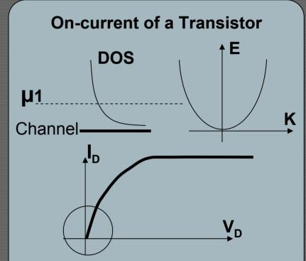
• Here, current flow depends on the availability of the states around the chemical potential. Higher DOS will result in higher current and low DOS will result in a small current. But why does the current saturate?
