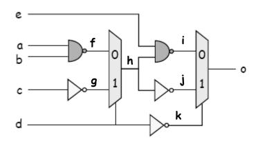
Delay(NAND2) = 2, Delay(INV)= 1, Delay(MUX) = 2
