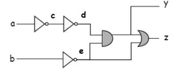
Delay(AND) = 2, Delay(INV)= 1, Delay(OR) = 2
