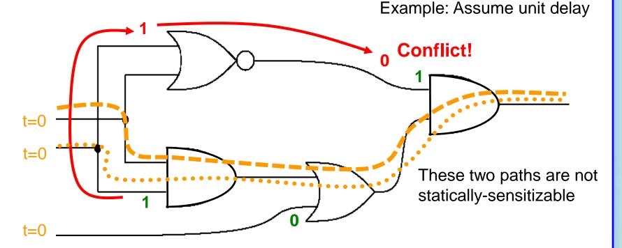
The longest statically sensitizable path is of length 2 Question: If inputs are applied at t = 0, does the output always stabilize by t = 2?
