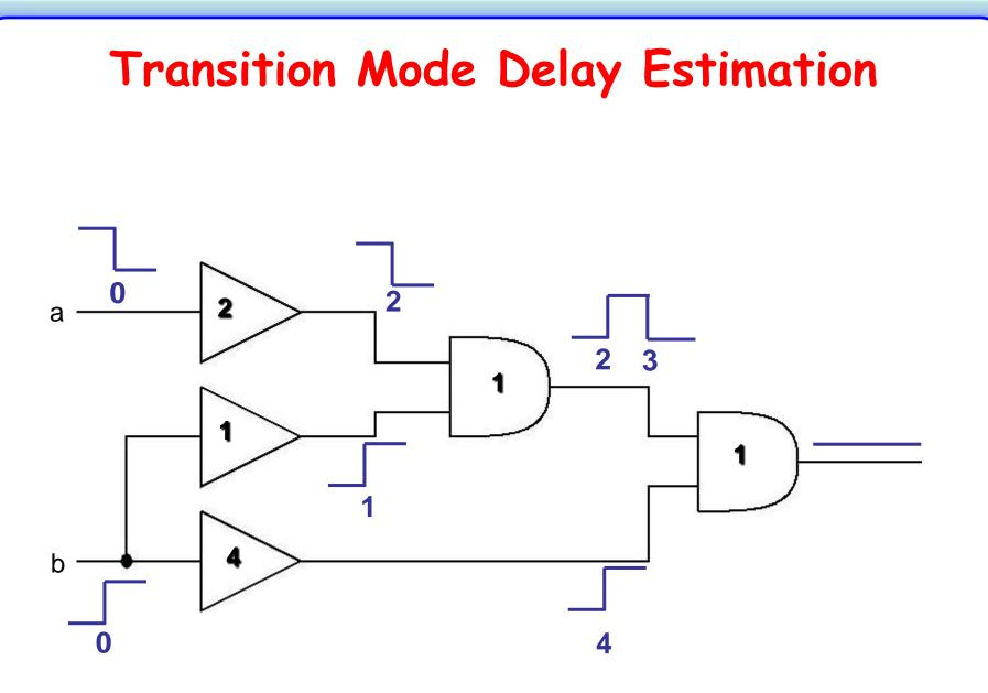
Output stabilizes at time t=0 under input vector pair a=1,b=0  $\rightarrow$  a=0,b=1
