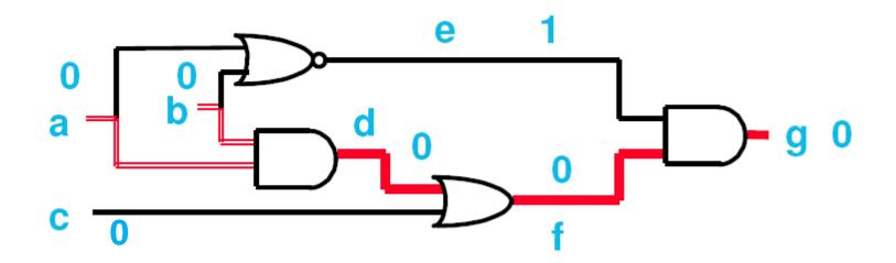
Paths  $a \rightarrow d \rightarrow f \rightarrow g$  and  $b \rightarrow d \rightarrow f \rightarrow g$  are co-sensitized by the input vector a=0,b=0,c=0
