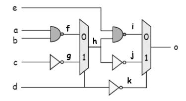
Delay(NAND2) = 2, Delay(INV) = 1, Delay(MUX) = 2
