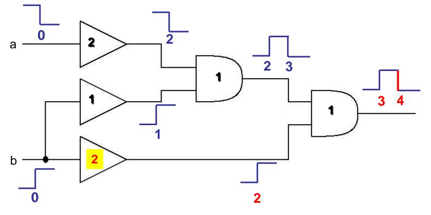
Output stabilizes at time t=4 under input vector pair a=1,b=0  $\rightarrow$  a=0,b=1
