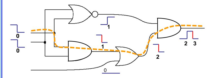
The longest statically sensitizable path is of length 2 Output stabilizes only at t = 3!
