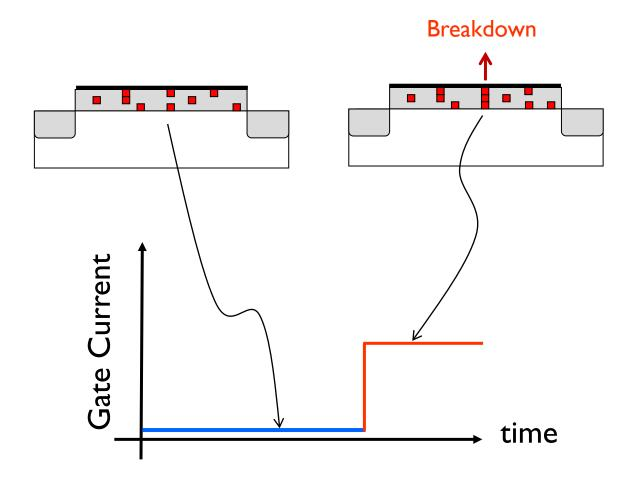
**Process:** Defect generation, Threshold: Breakdown
