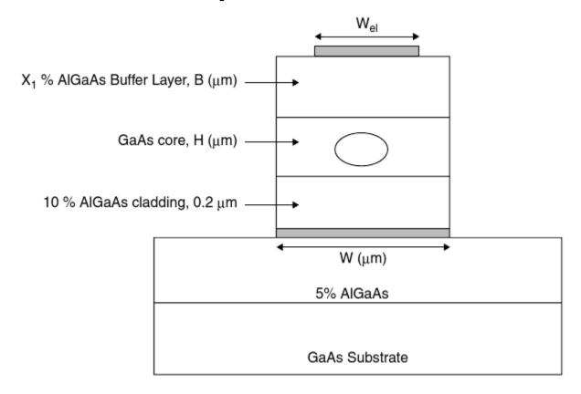
Schematic diagram of the electro-optic modulator, made from epitaxial GaAs/AlGaAs layers
