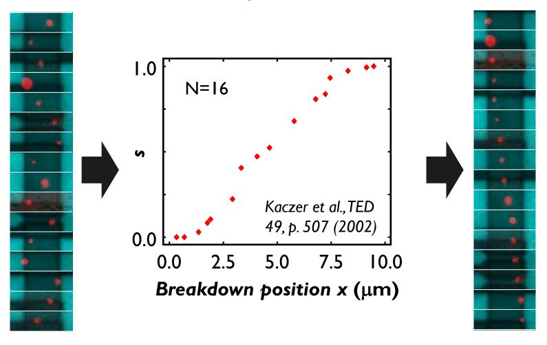
Emission microscopy on  $L=10 \mu m$  nFETs confirms the BD position determination method.
