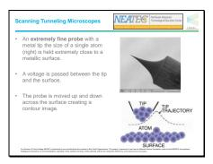
Slide 23 + 24: Simple overview of how a Scanning Tunnelling Microscope (STM) works. Here you can talk about the main difference between the two techniques i.e. AFM uses a needle to contour the surface; STM uses a current.
