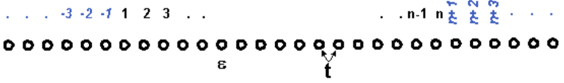
FIG. 6: A one dimensional device connected to two semi-infinite leads. While the potential in the leads are held fixed, the potential in the device can spatially vary.
