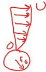
$$F_D = \underbrace{4\pi\mu U r_0}_C + \underbrace{2\pi\mu U r_0}_P = 6\pi\mu U r_0 \quad (\text{no slip})$$
