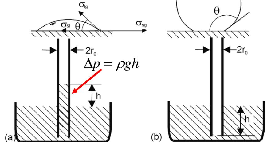
Capillary force driven pumping: (a) hydrophilic; and (b) hydrophobic.
