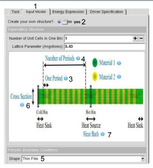
To simulate longer SiGe structures, as used in the paper, go back to the "Input Model" tab (1) and click "Create your own structure" (2)
