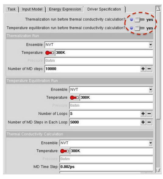
Unlike the prebuilt structures, every newly generated structure needs to undergo thermalization and temperature equilibration as part of the simulation, so these options should be switched to 'yes' under the "Driver Specification" Tab
