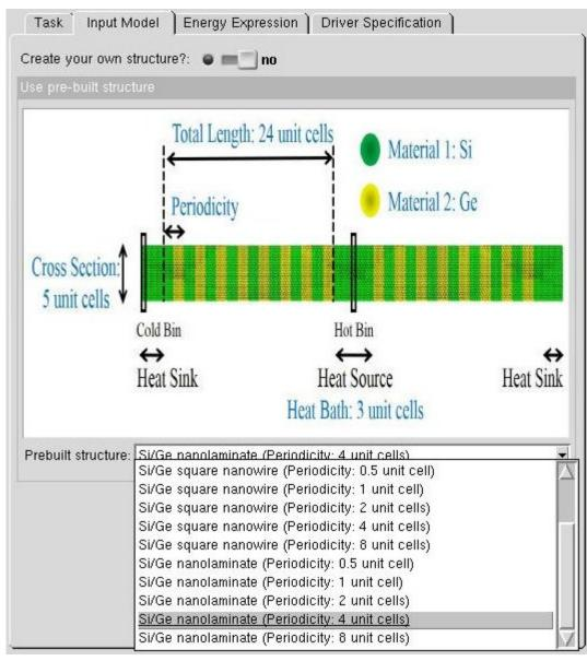
The tool supplies prebuilt structures for square nanowire and nanolaminate simulations
