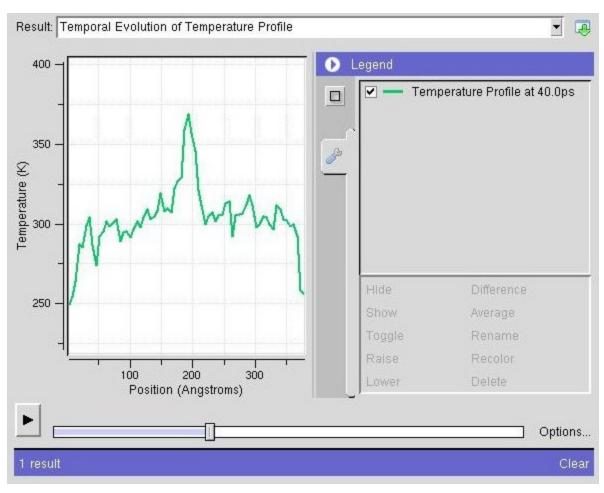
The "Temporal Evolution of Temperature Profile" page depicts the temperature profile of the specimen at periodic timesteps, which can be set as one of the simulation parameters. The slider at the bottom is used to cycle through the profiles
