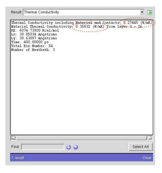
The "Thermal Conductivity" page gives the κ values for the material with contacts and for just the material
