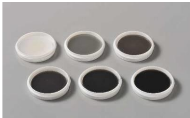
PE Resin Standard Samples Containing the 8 Controlled Elements in Toys
