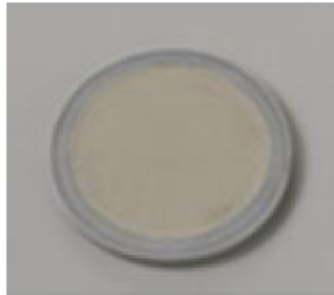
Fig. 1 Pressure-Formed Briquette of Cement
