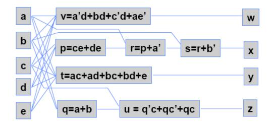
p = ce + de q = a + b r = p + a' s = r + b' t = ac + ad + bc + bd + e u = q'c + qc' + qc v = a'd + bd + c'd + ae' W = v x = s y = t z = u
