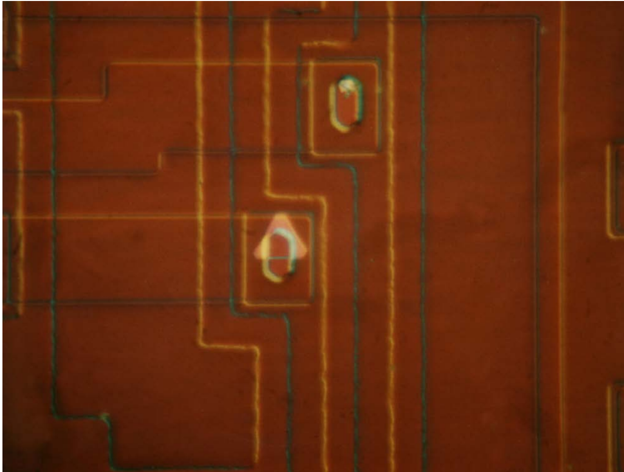
Aluminum-Silicon alloying pit made visible via Nomarski DIC
