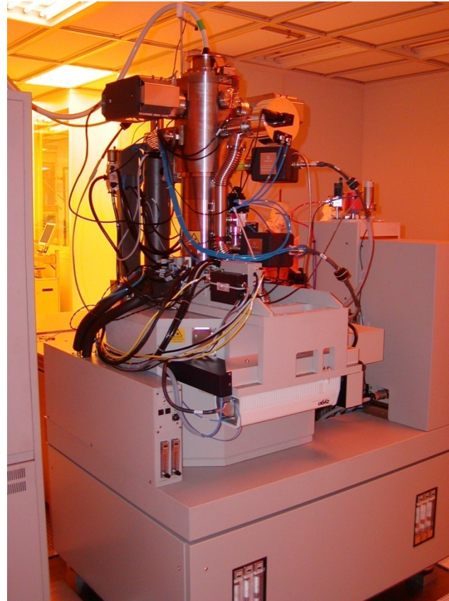
Temperature stabilized column, chamber and air lock
