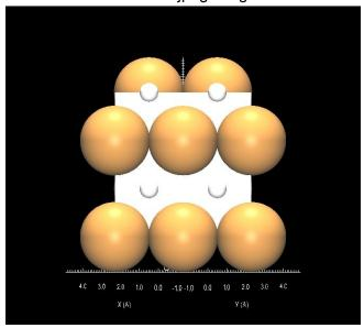
In this image, you see the (110) plane in white, with the 6 Cu atoms that are sitting on this plane. Ignore the small white spheres, they are artifacts of the program and needed to draw the plane and cut the structure, but are not atoms or part of the structure.
