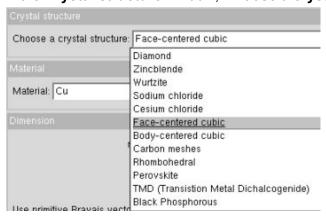
5. Use the default **Material**, **Cu** (Copper). Copy down the unit cell parameters that are provided. Be sure Draw miller plane is set to **no** to be able to see all of the information. Copper is a cubic crystal, so a1=a2=a3= 0.361 nm in the conventional unit cell.
