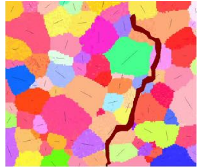
Numerical crack path (Basal trace of each grains are shown)
