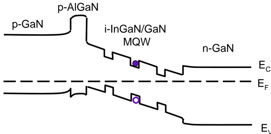
Typical band diagram at zero bias for a visible nitride LED
