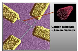
Nanotube connectors for microelectronics [University of California – Berkeley, Image source: Office of Basic Energy Sciences, U.S. DOE]
