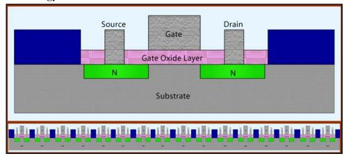
The space of one transistor, now holds hundreds of transistors (graphic not to scale)
