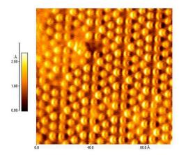
This atomic force microscope image by German physicist Franz Giessibl shows dozens of silicon atoms. Scientists have debated whether the light and dark crescents - or wing-shaped features seen on the atoms represent orbitals - the paths of electrons orbiting the atoms. [Printed with permission. See F. J. Giessibl et al., Science 289, 422 (2000)]
