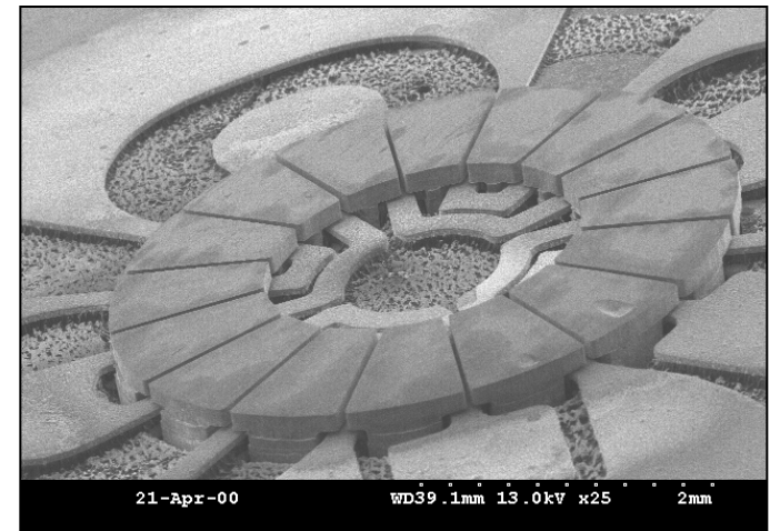
Electroplated NiFe core and Cu windings in a planar induction motor [Cros et al., 2004]
