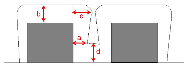
Sidewall Step Coverage= 100 x a/b (%)Bottom Step Coverage= 100 x d/b (%)Conformality= 100 x a/c (%)
