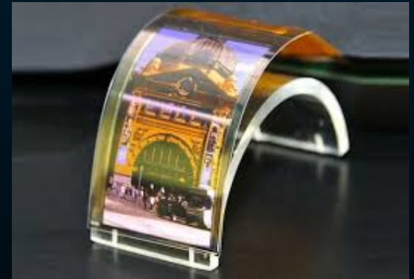
IGZO-based highly resolved flexible screen
