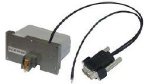
NT-MDT S.I. insert for SThEM measurement
