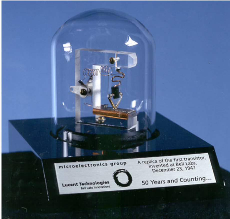
The first point contact transistor invented by Bardeen and Brattain at Bell Labs in 1947
