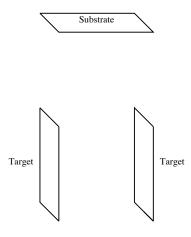
Nippon Steel developed the Facing Target Sputtering method, pictured schematically above, to generate Y-Ba-Cu vapor mixture which reacts with an oxygen atmosphere to deposit a thin film of  $YBa_2Cu_3O_7$  high-temperature superconductor on the substrate.
