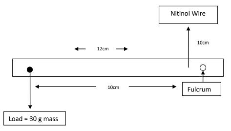
Connect the power supply to the each end of the nitinol wire with alligator clips. You will want to measure the current in the circuit with an ammeter and the voltage across the wire. Attach the leads of the voltmeter to the ends of the wire. Attach the leads to the alligator clips that are on the ends of the wire, not the wire itself.
