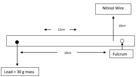
The nitinol wire is connected a distance from the fulcrum of approximately 1 cm. The load is attached 10 cm from the fulcrum. The lever should be 12 cm long with the fulcrum placed 1 cm from the end of the lever. The load should be a 30 gram mass
