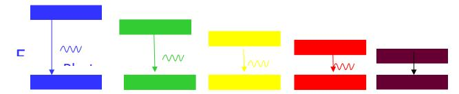
Bluer LEDs will excite a voltge in blue LEDs and other color LEDS towards the lower photon energy (redder) areas of the spectrum. (The dark red gap at the right of this picture is used to represent the nonvisible infrared LED which can be used.)
