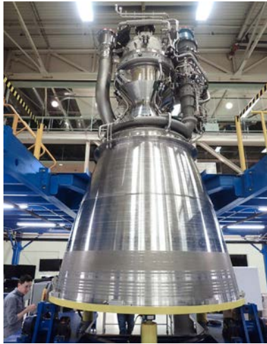
BE-4 rocket engine ( Blue Origin )
