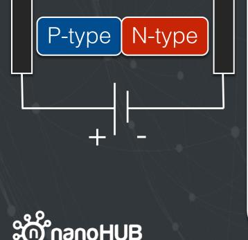
A PN junction is a device formed by combining p-type (doped with B, AI) and n-type (doped with P, As, Sb) semiconductors together in close
