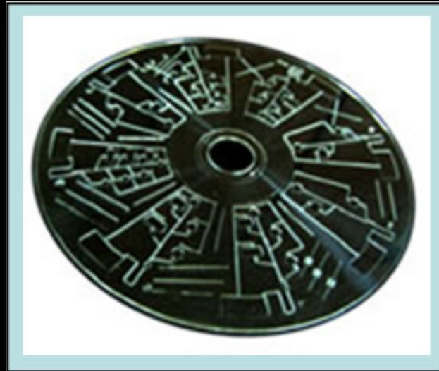
BioLOC's CD-Enzyme Linked Immunosorbent Assay - ELISA (ELISA™ – Printed with permission from BioLOC)
