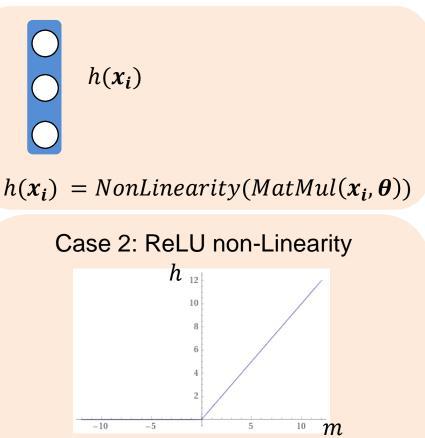
Saturation at **both** limits leads to bad gradients One limit is not saturated, better gradients
