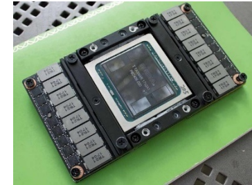
NVIDIA Volta GV100 (Graphics processor with 5120+640 "cores") 21 Billion transistors (12 nm)
