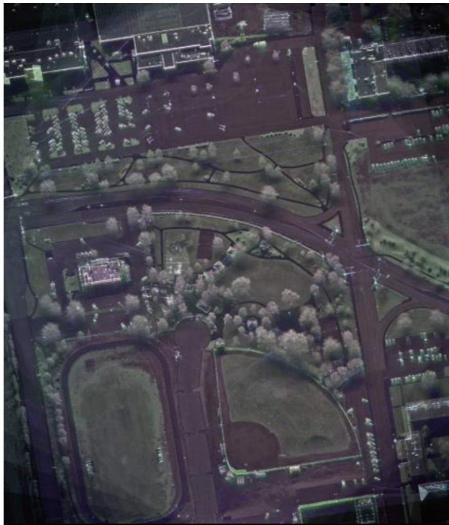
Figure 1.37: Example of a polarimetric SAR image of some buildings, parking lots, and New Mexico terrain. The coloring is done through processing of the polarization information received by the radar. Courtesy of Sandia National Laboratories, Radar ISR.
