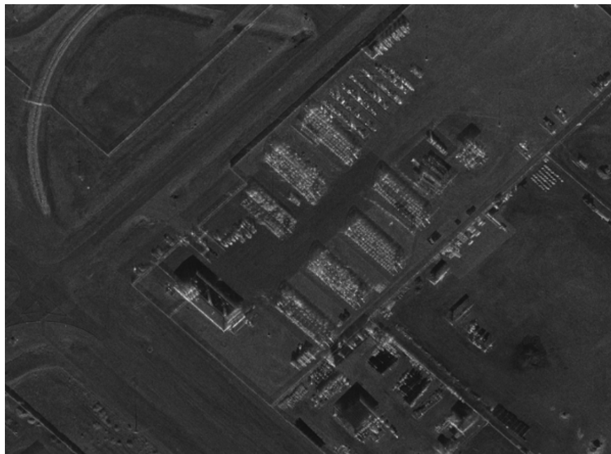
Figure 1.36: Example of a traditional “spotlight mode” SAR image of some buildings, parking lots, and New Mexico terrain. Courtesy of Sandia National Laboratories, Radar ISR.
