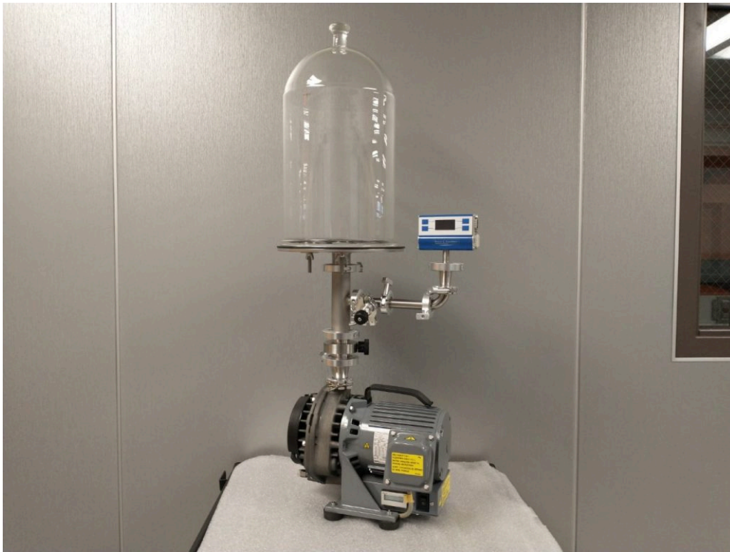
Figure 3.17. A simple rough-vacuum pumping system. Photo provided by Richard Hill, SUNY Erie Community College.
