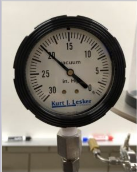
Figure 4.14.a. Bourdon gauge measurement of pressure inside a vacuum chamber. Photo provided by Nancy Louwagie, Normandale Community College.
