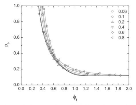
Fig. 8. The bond percolation threshold as a function of the total volume fraction for different values of  $\varepsilon$  indicated in the figure. The solid lines represent fits to equation (2) after transformation of  $\phi_e$  into  $\phi_t$ .
