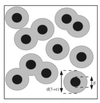
Fig. 1. Schematic representation of hard spheres with permeable shell. The black areas represent  $\phi$  and the sum of black and grey areas represents  $\phi_e$ .
