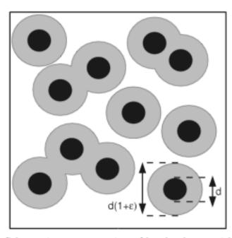
Fig. 1. Schematic representation of hard spheres with permeable shell. The black areas represent  $\phi$  and the sum of black and grey areas represents  $\phi_e$ .
