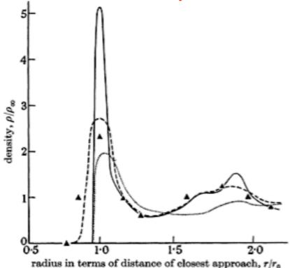
Figure 1. Radial distribution functions: variation of mean particle density as a function of  $r/r_0$ . ....., Derived from calculated random model; -----, derived from squeezed random model; -----, calculated for liquid lead by Furukawa (1960) with X-rays calculated for liquid argon by Henshaw, D. G. (Phys. Rev. 105, 976; 1957) with neutron diffraction.
