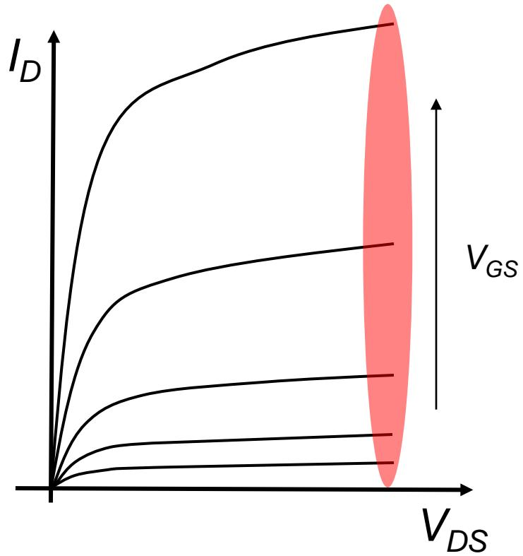
$$I_D = \frac{W}{2L_{ch}} \mu_0 C_{ox} \frac{(V_G - V_{th})^2}{m}$$
