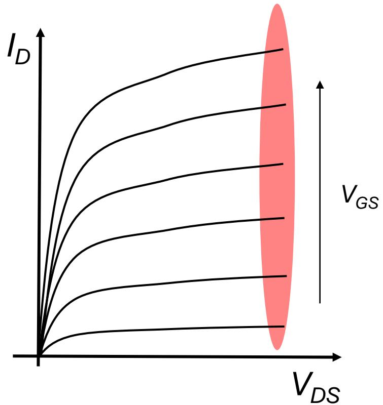
$$I_D(V_D = V_{DD}) \sim (V_G - V_{th})^\alpha$$
