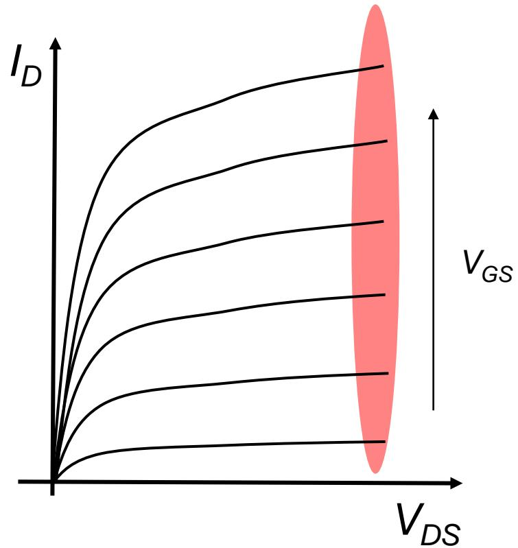
$$I_D = W v_{sat} C_{ox} (V_G - V_{th})$$
