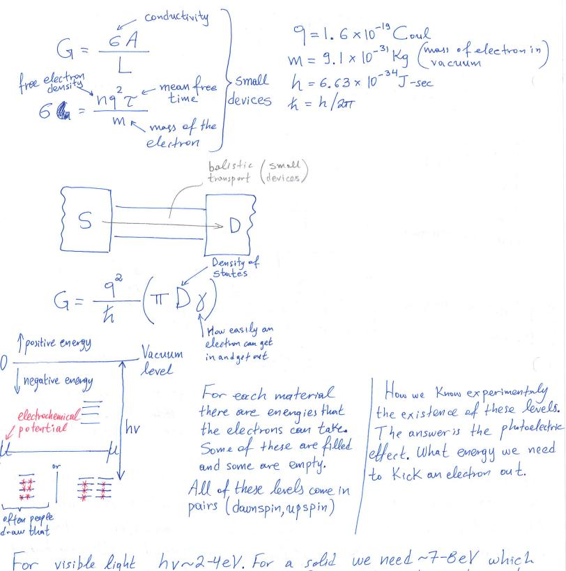
For visible light hv~2-4eV. For a solid we need ~7-8eV which means that this light is not visible. But photo-emitions does not give information for the empty states. For these energy we have the absorption of light.
