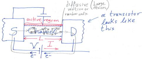
if we apply a positive voltage then electrons will move as shown in the figure that above. The direction of current has opposite direction because the electrons have negative charge.
