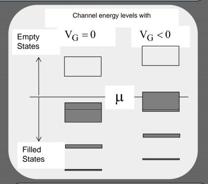
• Apply a *positive* gate voltage and band energy levels move *down*.
