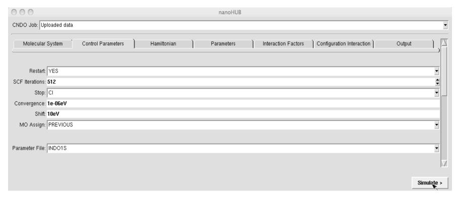
Figure 11: Restarting incomplete SCF calculations. Set *Restart*: YES and *MO Assign*: PREVIOUS.
