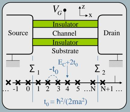
• Last time we discussed the change in the electron density due to the gate voltage. As VG changes the levels in the channel move up and down.
