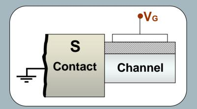
• In this the electrons can from a continuum of allowed states in the contact want to get into the channel. The governing equation for the channel can now be written as:
