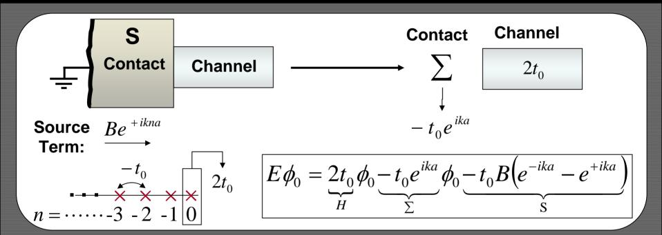
ullet One main difference between H and  $\Sigma$  is that the diagonal elements of  $\Sigma$  are complex in general whereas H has real values for its diagonal elements because it has to be Hermitian.
