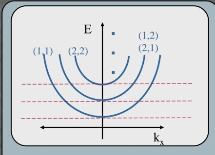
Notice that for a bigger cross section the bands get closer to each other. As the result the number of modes in the energy range of interest will increase and the resistance will decrease. Higher cross section → Lower resistance.
