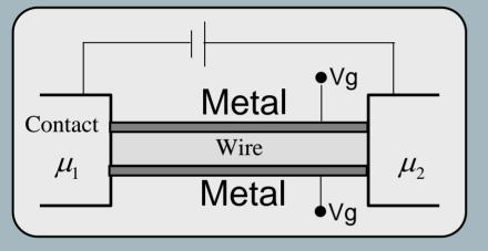
• The voltage applied to the metals could actually deplete the wire and make the effective cross section smaller.
