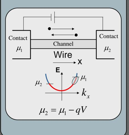
• The current in this wire can be calculated  $I = \frac{2q}{h} (\mu_1 - \mu_2) \Longrightarrow$ as:  $G_{\max} = \frac{I}{V} = \frac{2q^2}{h} = 80\frac{\mu A}{V}$  $R_{\rm min} \approx 12.5 k\Omega$ • For several modes:  $R_{\min} \approx [12.5 / M] k\Omega$ Positive current E' Available carrying states and Conducting conducting modes Modes Ц  $\mu_2$ k<sub>x</sub>
