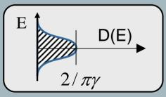
For weak coupling the channel only responds at certain sharp energies. For strong coupling the levels broaden out and the channel responds at more energy values because of broadening.
