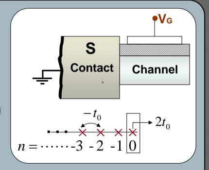
• Here, H describes the channel. Sigma describes the surrounding. "S" is the source term which tells us how electrons are getting into the channel. "S" is what drives the channel. psi is the response of the channel to the excitation by the contact. DOS tells us how well the channel responds at a given energy.
