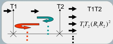
$$T = T_1 T_2 (1 + x + x^2 + ...), x = R_1 R_2$$
