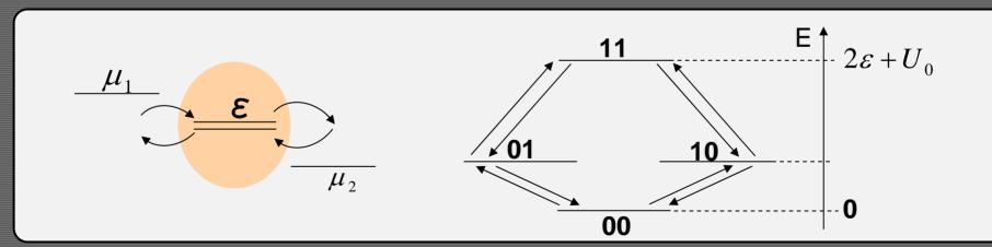
• In general we have 2^N sates for multi electron system where N is the number of allowed energy levels for the electrons in the device.
