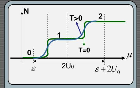
• You can see from the figure above that when T is large (for example room temperature) the smoothed curve above will actually be very close to the Self Consistent Field (SCF) curve drawn on the left figure. Under this conditions coulomb blockade cannot be observed.
