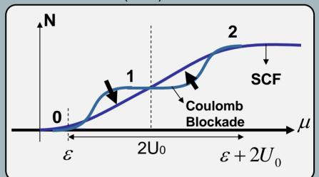
• So as long as  $\gamma, k_BT << U_0$  is **NOT** the case we get the correct results if we use the SCF method as before.
