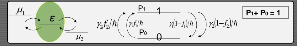
• At steady state, the rate at which an electron comes in must be equal to the rate at which electron goes out; therefore:  $P_0R_a=P_1R_b$
