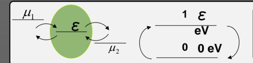
• When an electron comes in, the system goes form state 0 to state 1. When an electron goes out, the system goes from state 1 to state 0.
