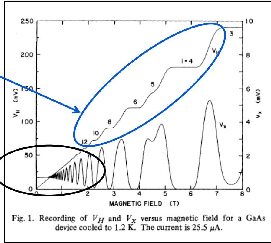
M.E. Cage, R.F. Dziuba, and B.F. Field, “A Test of the Quantum Hall Effect as a Resistance Standard,” *IEEE Trans. Instrumentation and Measurement*, Vol. IM-34, pp. 301-303, 1985
