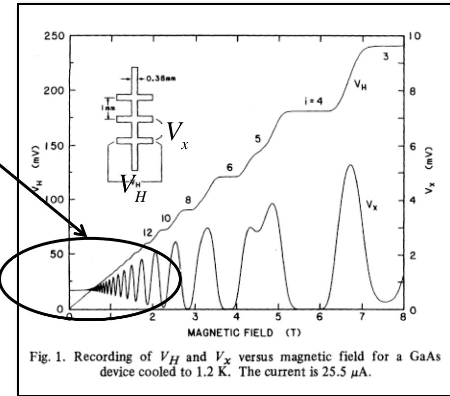
M.E. Cage, R.F. Dziuba, and B.F. Field, “A Test of the Quantum Hall Effect as a Resistance Standard,” *IEEE Trans. Instrumentation and Measurement*, Vol. IM-34, pp. 301-303, 1985
