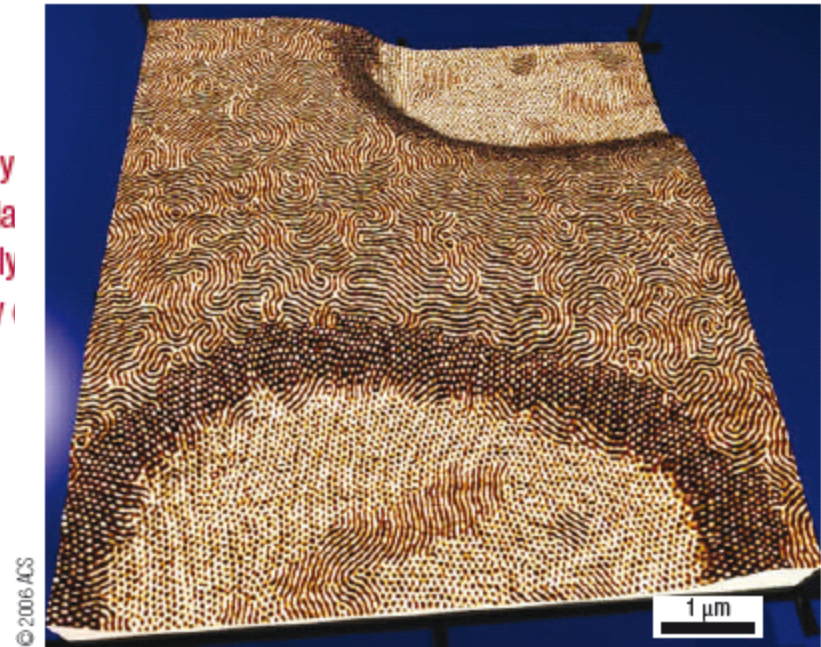
Figure 4 Complex microdomain structure of a block copolymer. The AFM images are rendered into three-dimensions using the height image as height-field and the phase image as contrast. The images show the formation of terraces in a thin film of SBS block copolymer and the systematic change of microdomain structures along the changes in film thickness from 32 nm at the lowest terrace to 57 nm at the higher terrace. Reprinted with permission from ref. 54.
