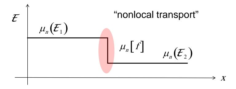
The concept of a field-dependent mobility applies <u>only</u> when the electric field changes slowly with position.
