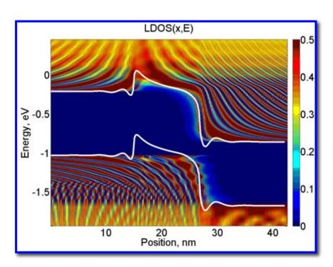
source + drain-injected LDOS in a carbon nanotube MOSFET
