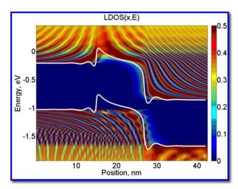
source + drain-injected LDOS in a carbon nanotube MOSFET
