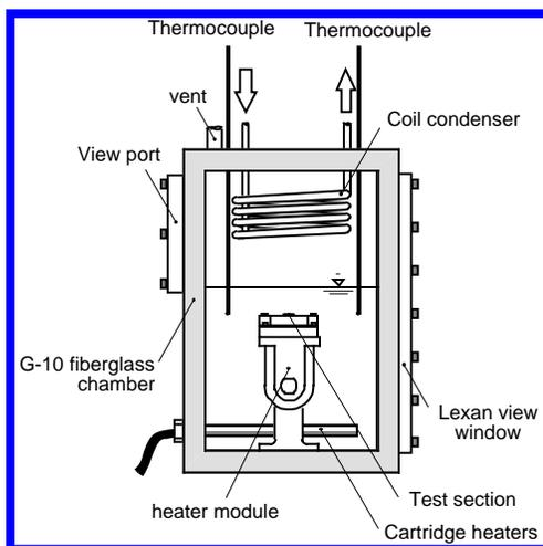
**Fig 2. Boiling Chamber**
